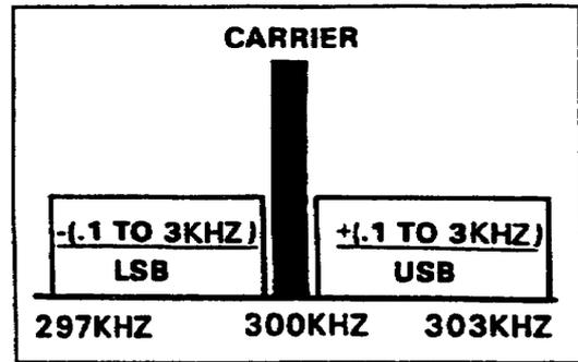
Figure 1-8. Amplitude-modulated system.
