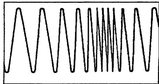
Figure 1-9. Frequency modulation.
