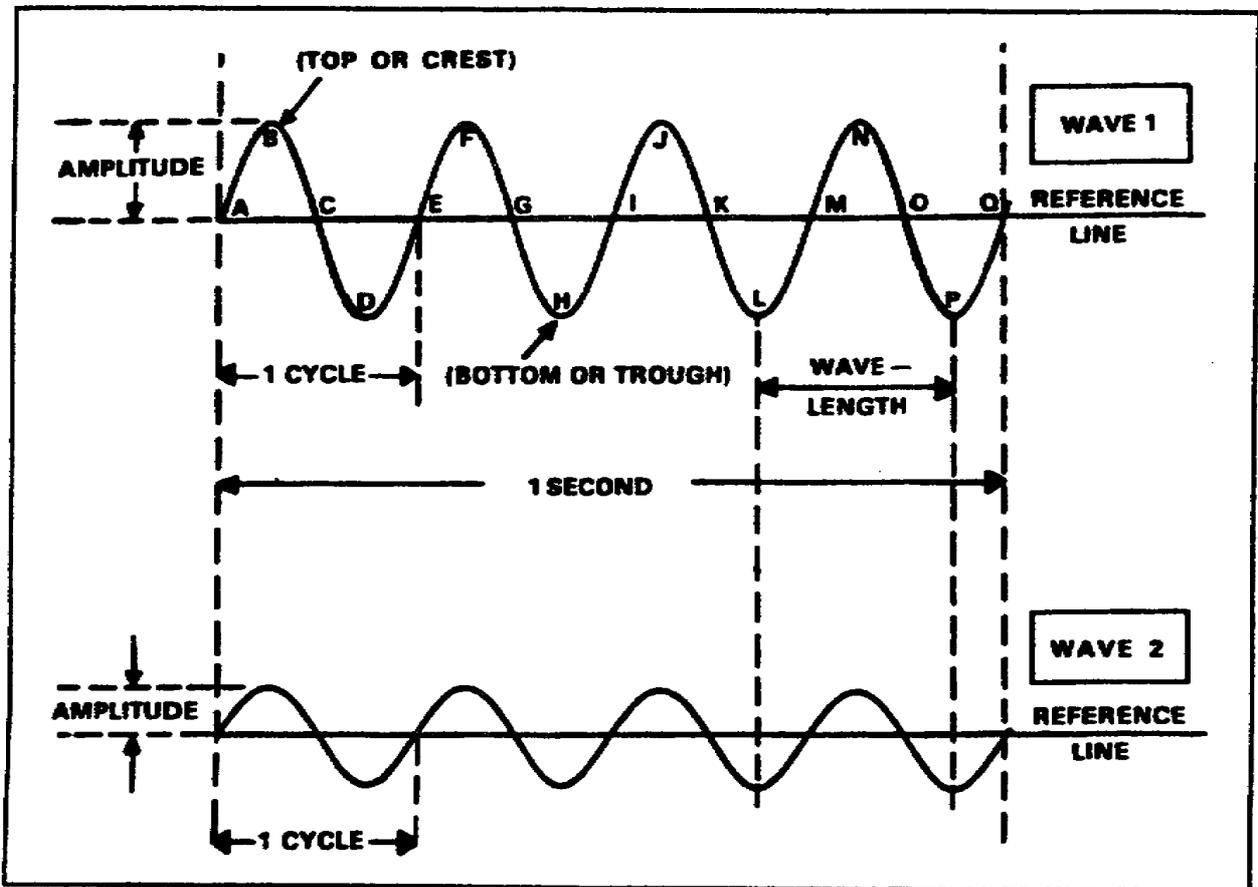
Figure 1-3. Comparison of waves with different amplitudes
