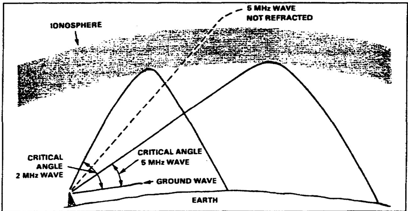
Figure 3-5. Effect of frequency on the critical angle.
