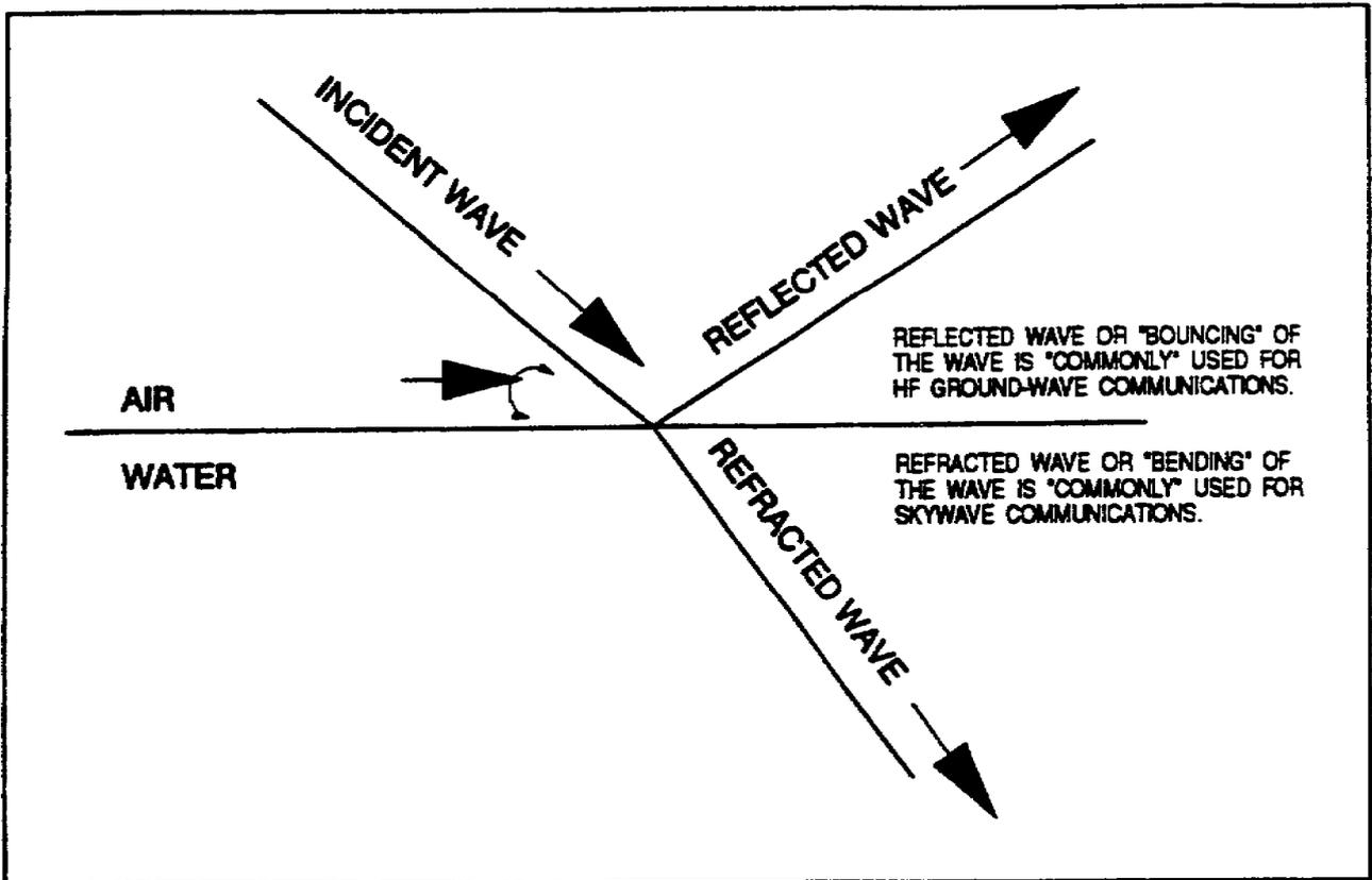
Figure 1-10. Reflection and refraction of a light beam.
