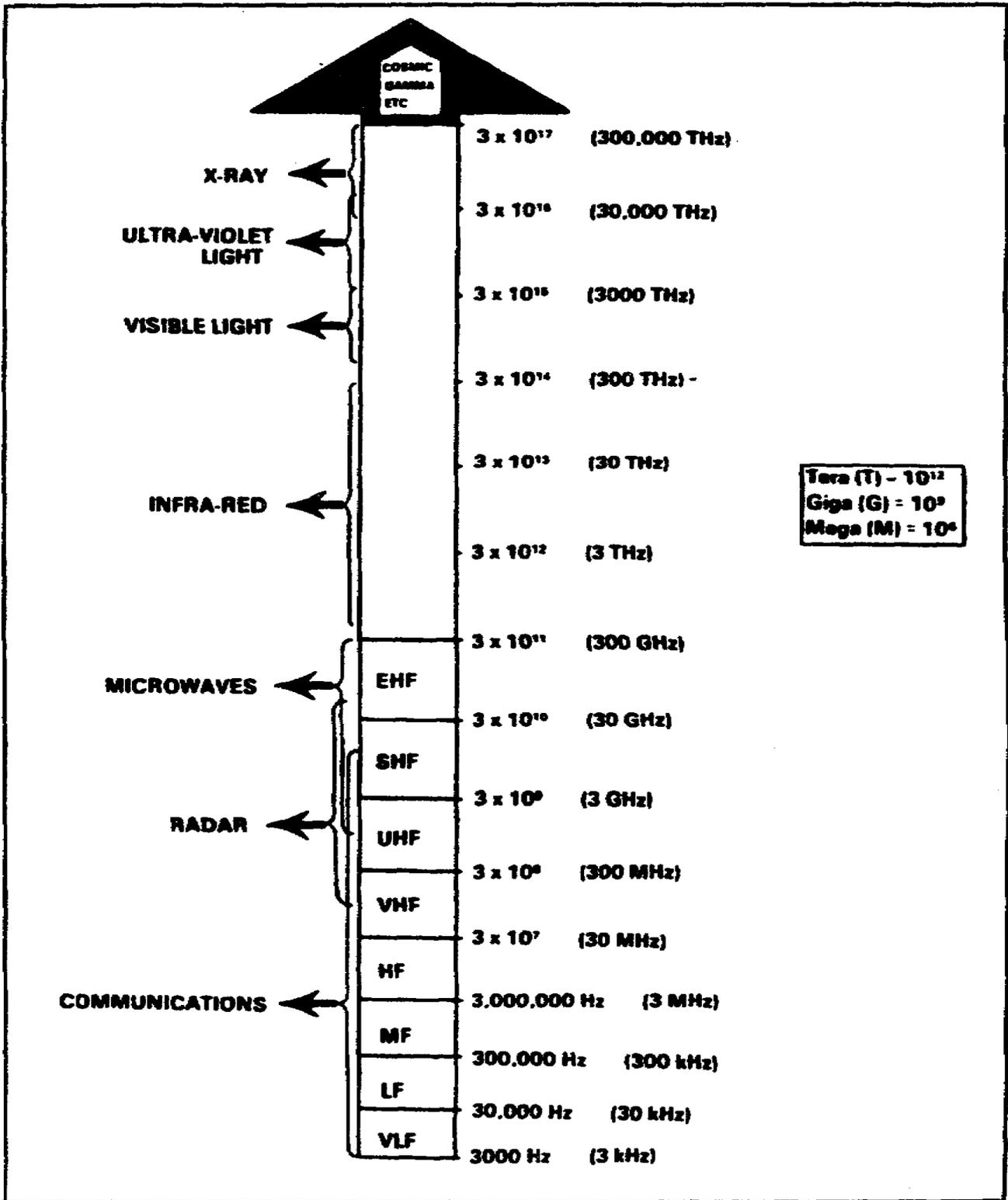
Figure 1-4. Electromagnetic spectrum.
