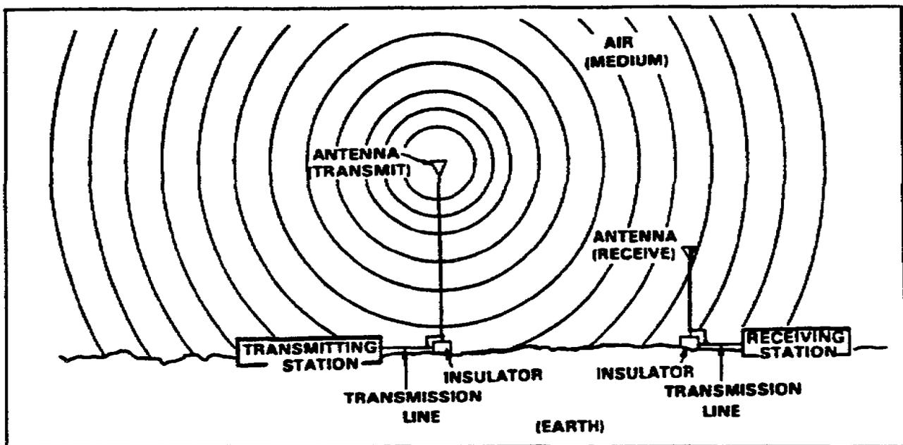
Figure 1-5. Simple radio communication system.
