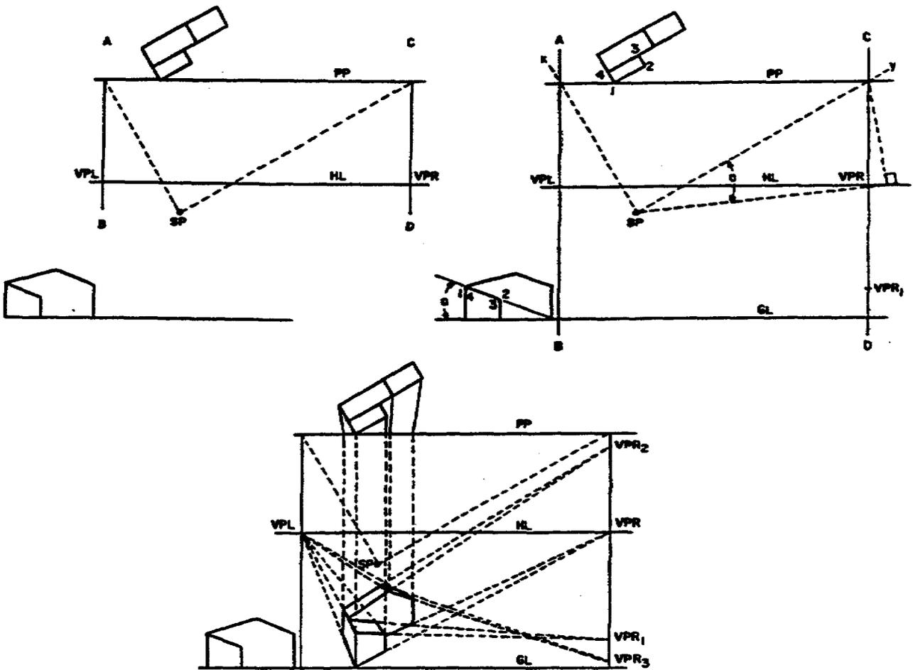
Figure 2-7. Finding the vanishing points for incline lines
