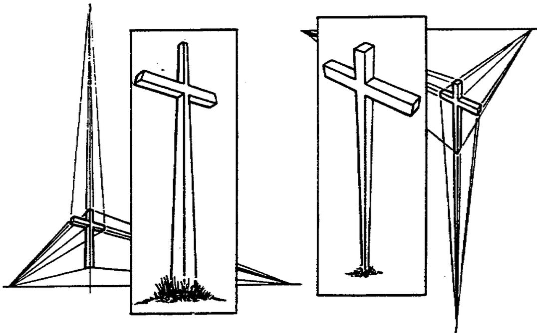
Figure 3-1. Three-point perspective
