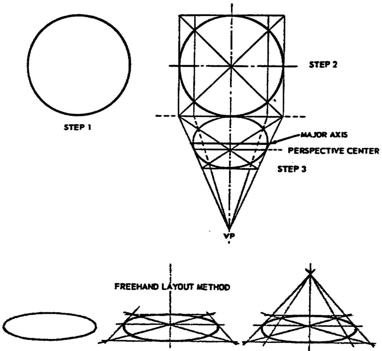
Figure 3-5. Mechanical tool and freehand layout methods
