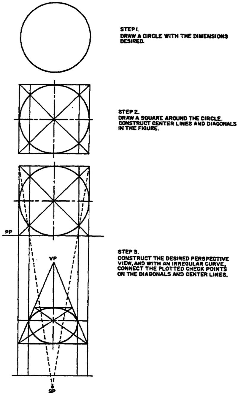
Figure 2-8. Layout for a circle in perspective
