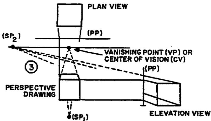
9. DRAW PERPENDICULAR PROJECTORS FROM BOTH PP'S TO LOCATE CORNER PLOTS OF THE OBJECT.
