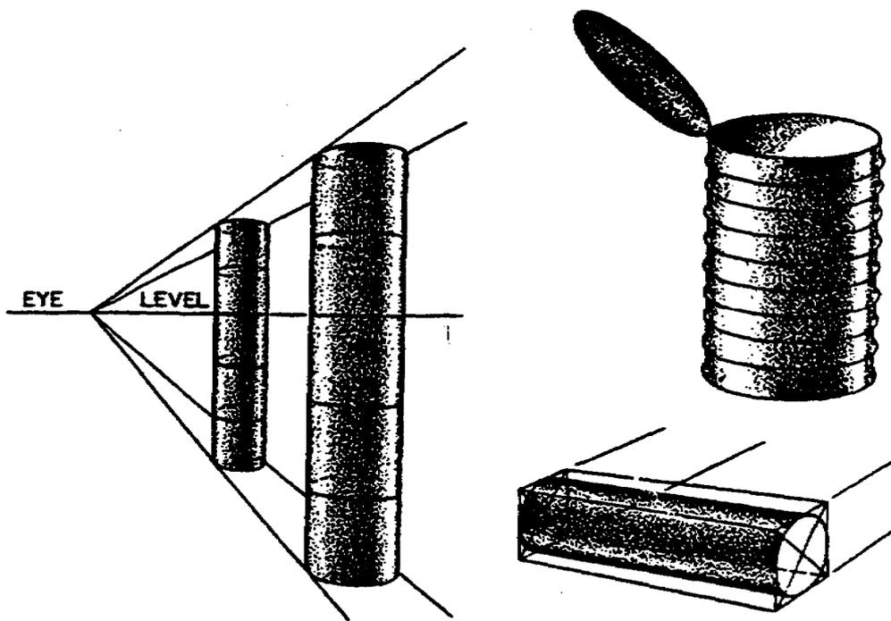
Figure 2-11. Perspective circles when in relation to cylinders
