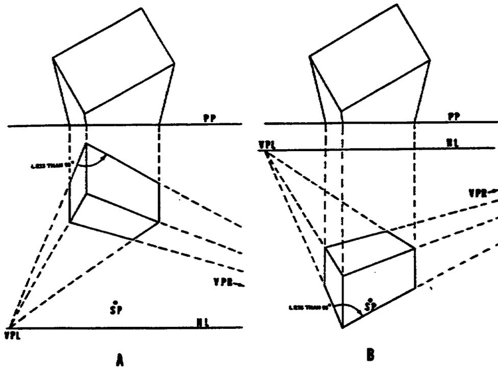
Figure 2-6. A. Object placed too high above eye level
