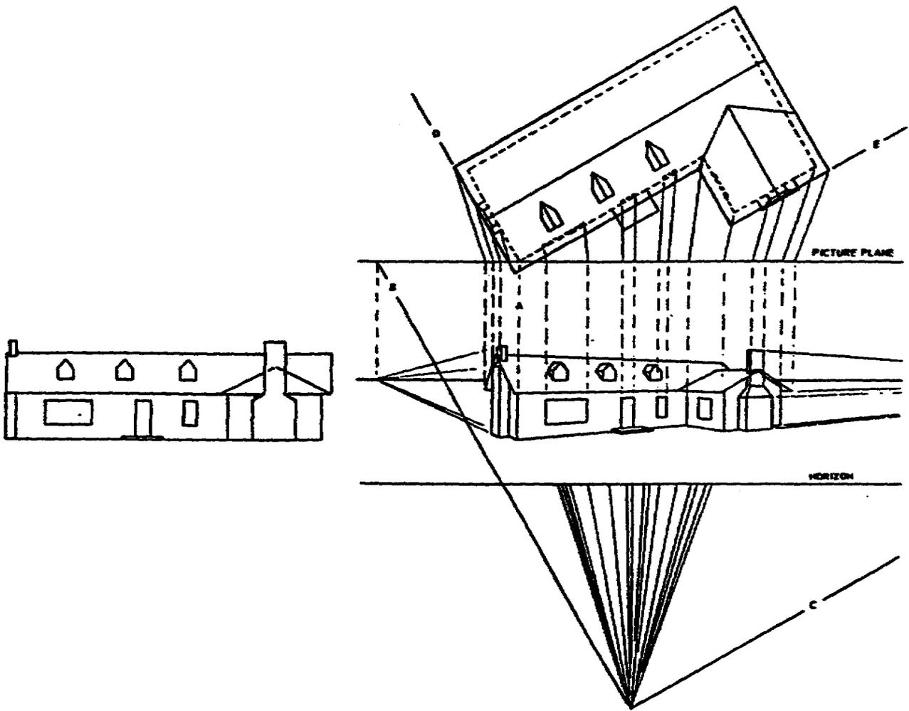
Figure 3-6. Plan and elevation views
