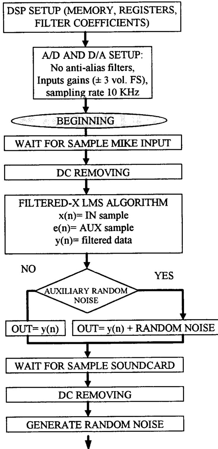
Figure 4. Programming structure of the active noise controller (continued)
